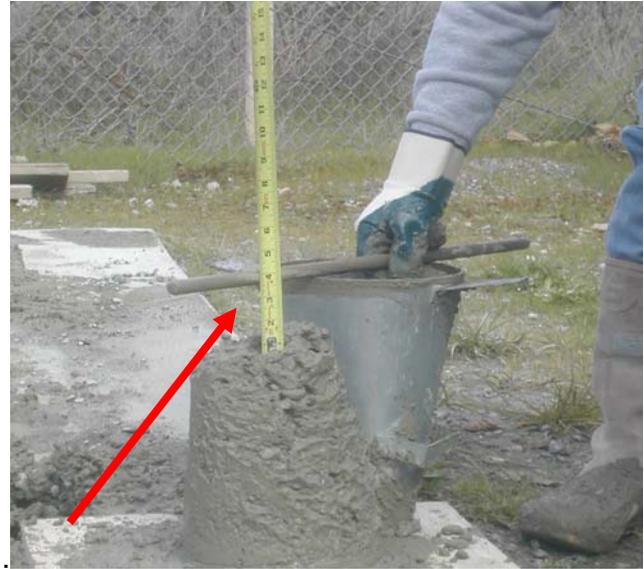
A 3" slump is measured here
