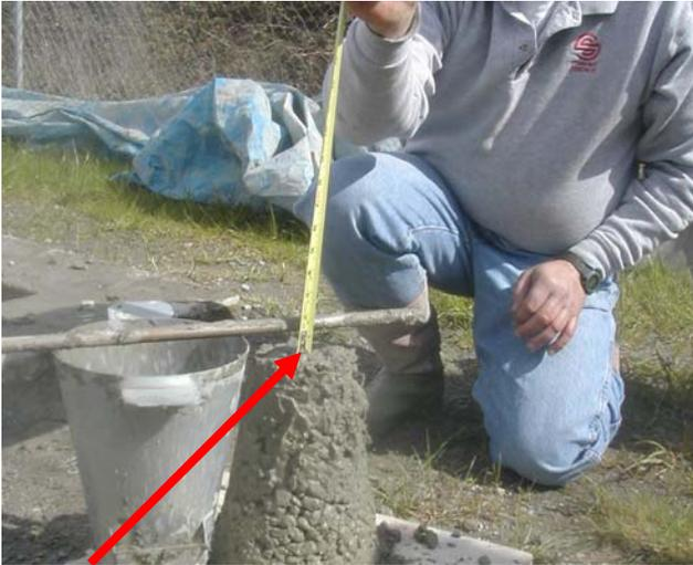
A 1" slump is measured here
