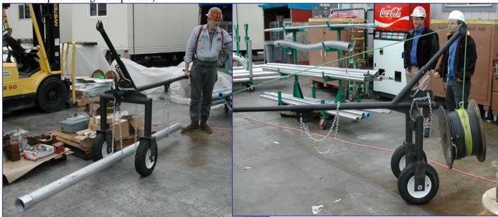
Shown next is the buggy being used to lift and transport a Walk-Behind Power Trowel used for finishing concrete. The combination of weight, (machines vary from 200 to 300 pounds depending on size) and the awkward shape for manual handling, make this type of task ideal for the buggy's intervention.
