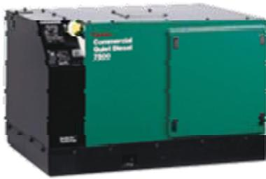
Newer heavy duty diesel generators are designed to emit low noise and vibration. Some units are up to 15 dB (A) quieter than older diesel-powered generators and quieter than most gasoline sets. The units are totally enclosed and damped, including cooling, exhaust and intake systems.
