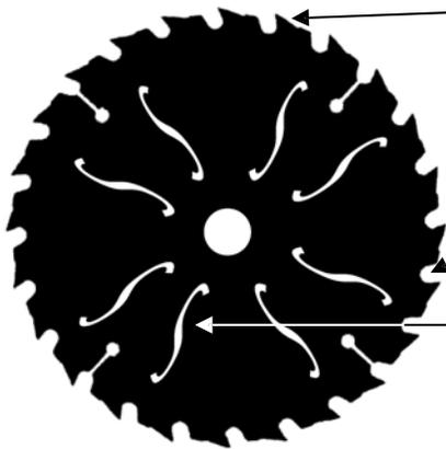
Choose a saw blade with the greatest number of teeth, of the smallest width
